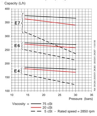
Data shown take into account a wear margin. Do not oversize the pump when selecting the gear capacity.
